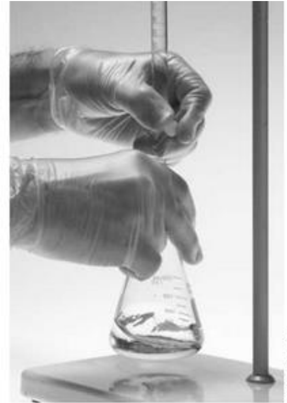
Figure 2-23 Recommended method for manipulating a buret stopcock.
